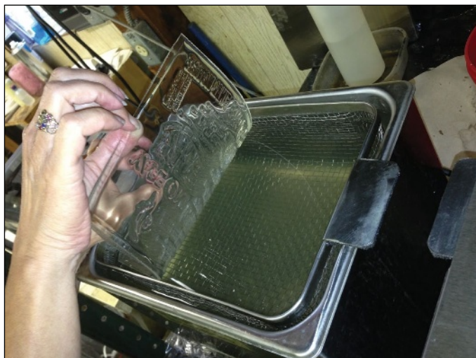
Exposed polymer plate being inserted into ultrasonic washout unit for removal of unexposed resin.
