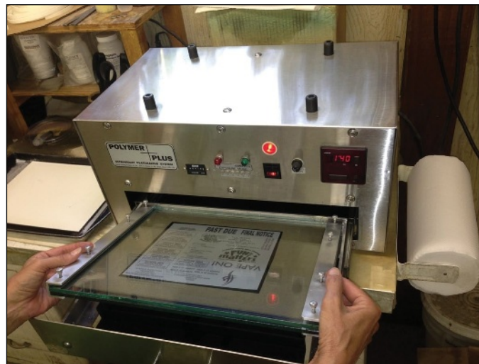
Laser printed vellum and negative film locked between glass plates and inserted into exposure unit.
