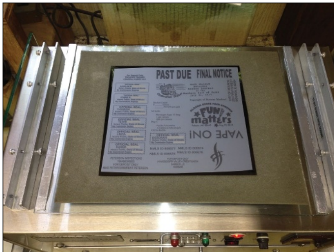
Laser printed vellum paper in contact with negative film before exposure.
