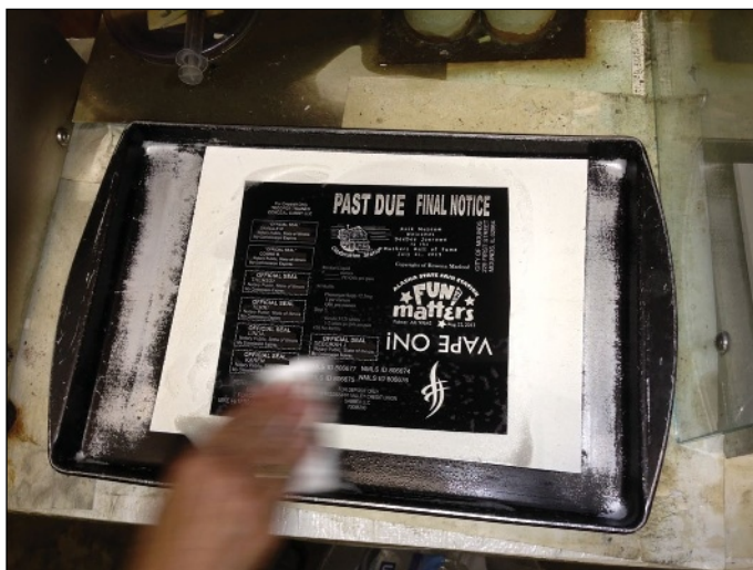
Developer solution applied to film and wiped with cotton pad to create reverse image negative.
