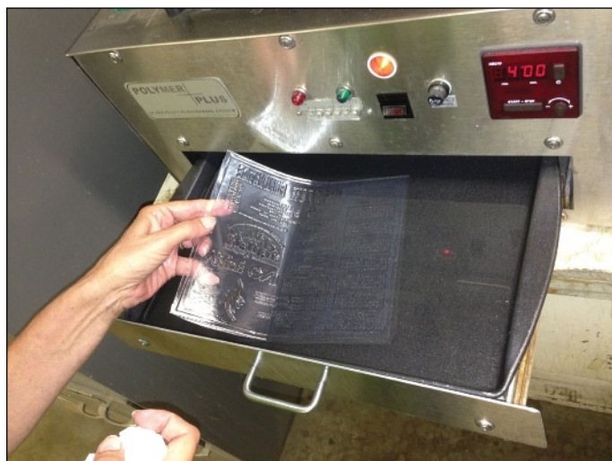
Washed polymer plate inserted into pan of water for post-exposure hardening in the exposure unit.
