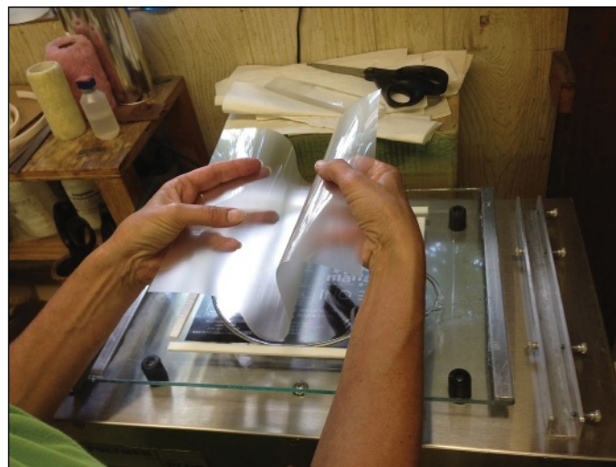
Applying substrate backing to the poured polymer.
