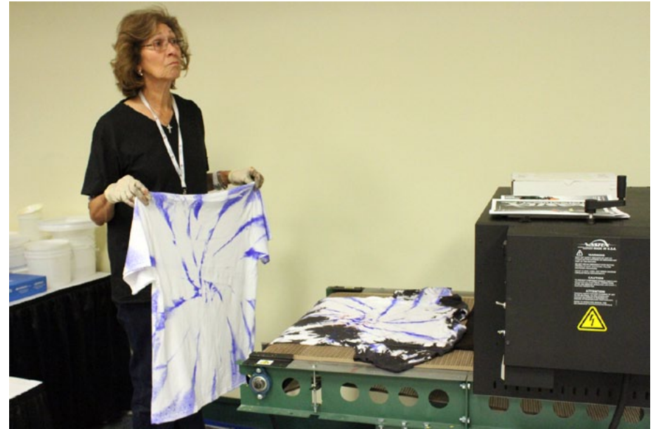
Once you're done spraying, run the shirt through a conveyor dryer. They also can be air dried.
