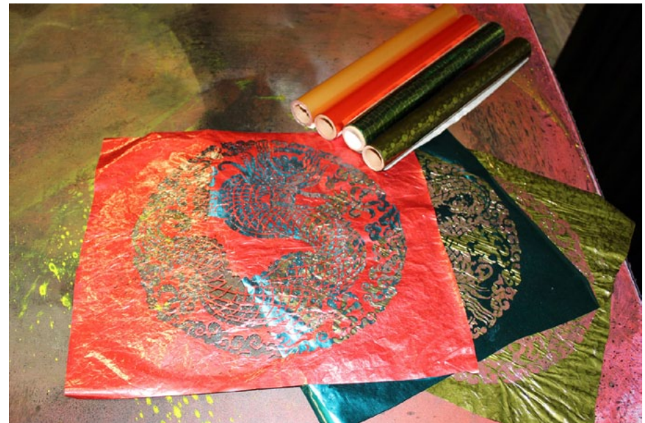
Foil adds bling to any design. This dragon was screen printed onto a shirt with foil adhesive. The shirt is then placed on a heat press and a sheet of foil is placed over the design. It is heat pressed to bond it to the shirt.
