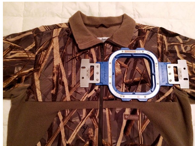
This is an example of a left-chest size hoop. You want to ensure there is a least a finger's width between the design and the edge of the hoop to avoid the needle hitting the hoop. Photo courtesy of GSG, Dallas
