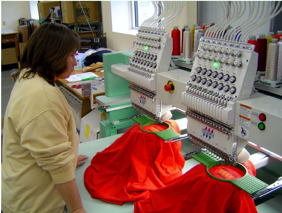
By choosing the right hoop for the substrate, you ensure the job will run smoothly and produce the highest quality result. Photo courtesy of Mind's Eye Graphics, Decatur, Ind.
